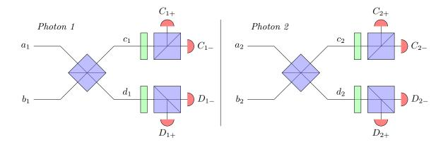
Here, blue squares represent polarising beam splitters (PBS) that transmit photons in  $|V\rangle$  and reflect photons in  $|H\rangle$  polarisation. Green rectangles represent half-wave plates (HWP) oriented at  $\pi/8$  angle, such that  $|H\rangle \to \frac{1}{\sqrt{2}} [|H\rangle + |V\rangle]$  and  $|V\rangle \to \frac{1}{\sqrt{2}} [|H\rangle - |V\rangle]$ . Red half circles represent single-photon counters.
