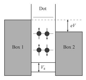
What condition has to be fulfilled that electrons can hop from the right to the left reservoir via the dot and when does the dot 'block'? Make a diagram with axes V and  $V_g$  showing regions where there is a current and regions where there's none.
