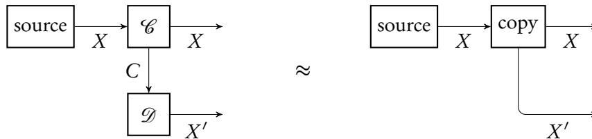
Figure 7.3: Data compression. The random variable C is the compressed version of X , since the decompressor \mathcal{D} can recreate the particular output of the source (stored in X ) from it.
