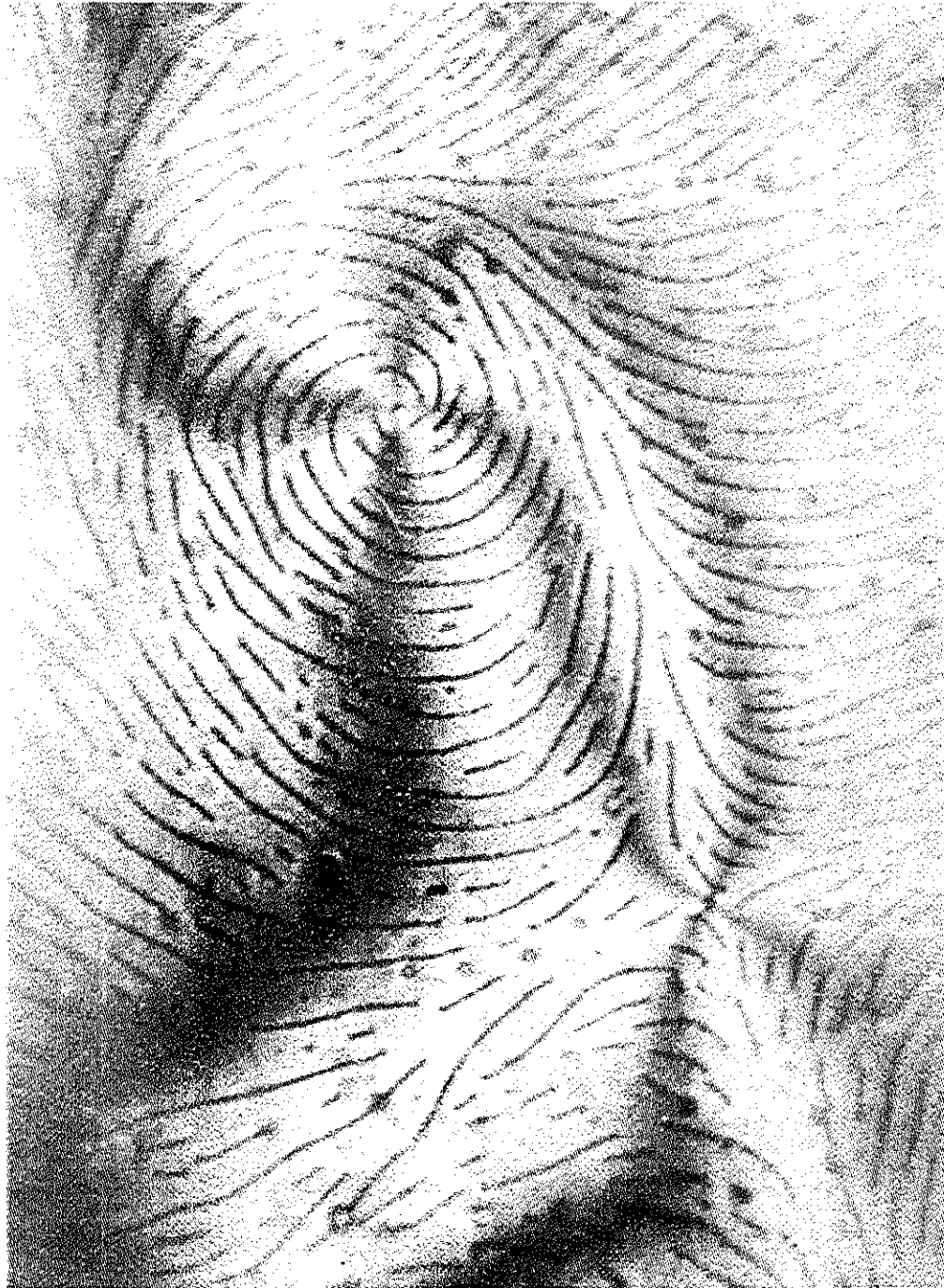
Fig. 4.4. Bubble decoration technique displaying the arrangement of the molecules at a free surface (courtesy P. Pieranski) [4]. In the present example we see two singular points of strength (+1) and (-1) between crossed polarizers.
